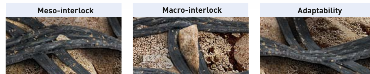
Meso-interlock Interlock between soil particles and geogrid ribs due to surface texture.
