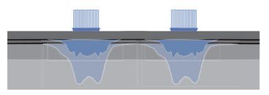
Tensile force distribution in the horizontal reinforcement layers (FEM)
