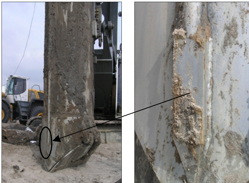
Figure 16. Displacement pipe equipped with measurement instrumentation to record acoustic signals
