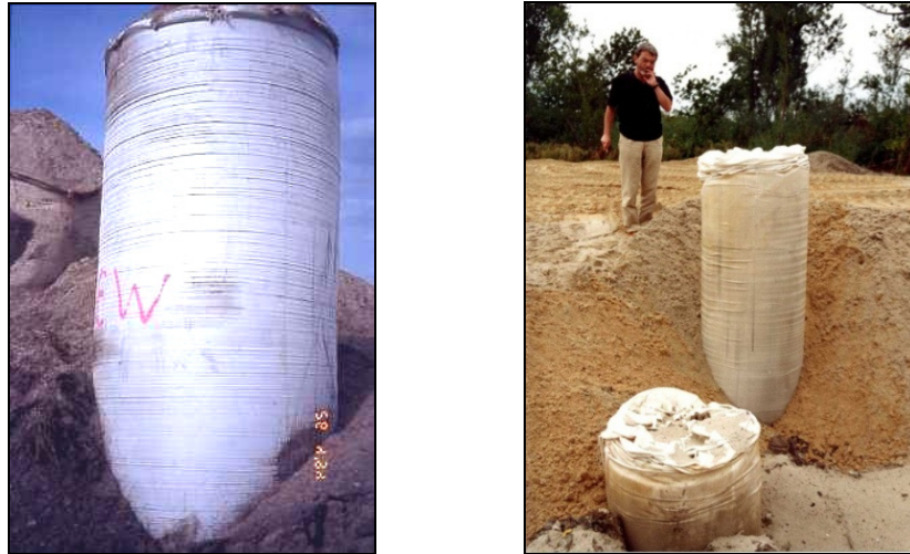
Figure 3. Demonstration of the confining capability of high strength geotextile encasement for GEC “in air”
