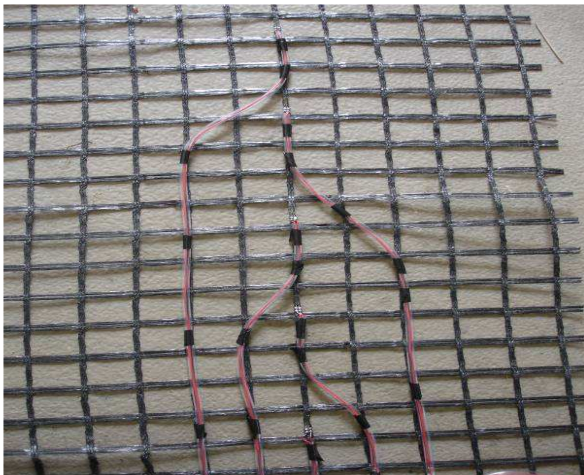
Fig. 4. Strain gage setup on geogrid
