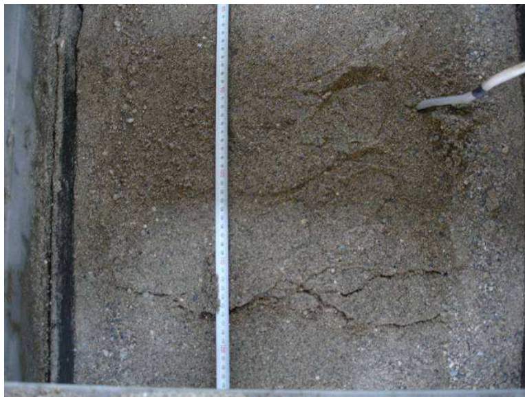
Fig. 7. Tensile cracks observed in sand backfill
