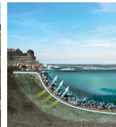
Isolation of contaminated sediments
