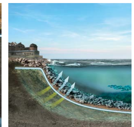
Isolation of contaminated sediments
