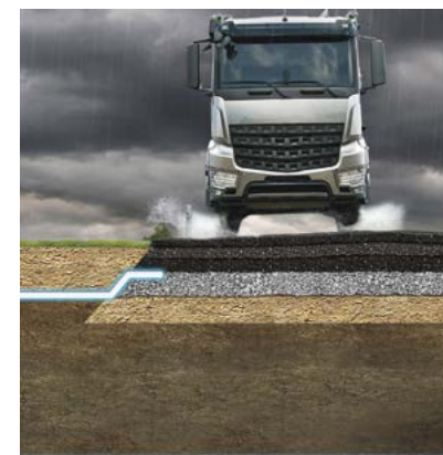
Decentralized runoff treatment on roads
