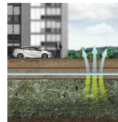
Soil air filter on contaminated sites
