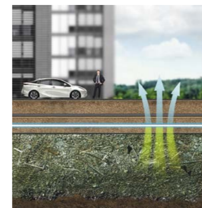
Soil air filter on contaminated sites
