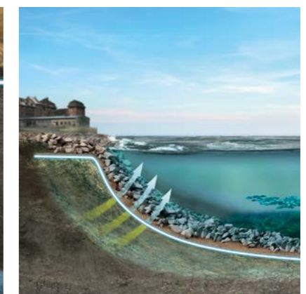
Isolation of contaminated sediments
